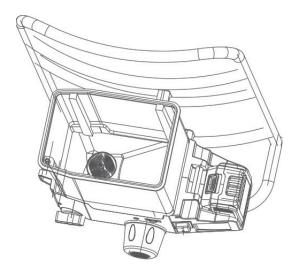
3. Remove the outlet valve, clean it and check if there is any damage, or replace the outlet valve.
