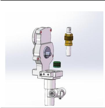
2. Put the piston rod into the pump body.
