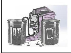
7. Turn pressure control knob counterclockwise to the Prime/Clean setting.
