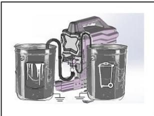
6. Turn Prime/Spray valve down to PRIME position.
