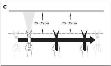
Press the spray gun trigger after starting the arm movement. Re lease the trigger before finishing the movement.
