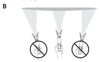
This means you have to move your whole arm back and forth instead of just the wrist. Hold the spray gun perpendicular to the surface; otherwise a part of the application area is painted thicker than with other parts
